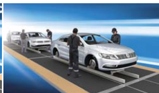
The Skid Transfer System
